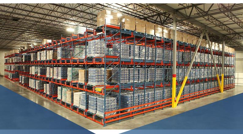
"What really drove the decision was how fast we could effectively load the system and offload to the truck with a limited number of operators. With a 25" deep, 40" wide Pallet Moleù system only feet from the bottling line and the loading dock, we are extremely confident that we'll reach our goal of twenty minutes per truck load in Kansas City."
